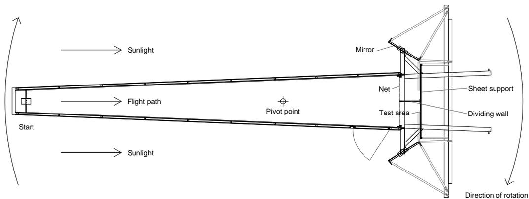
Figure 2: Horizontal section through the Flight Tunnel II in the ONR test configuration. The entire tunnel is mounted on a pivoting device and is turned clockwise to follow the position of the sun. Thus, the direction of sunlight is always parallel to the birds' line of flight. The test area is illuminated with natural (sun)light via two lateral mirrors.
