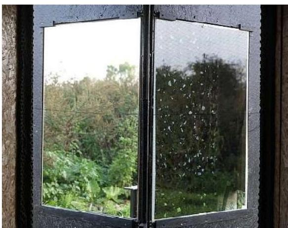
Figure 12: WIN test (WIN 2014). Mirror on the left (reference), test pane on the right (*birdpen* on float glass)
