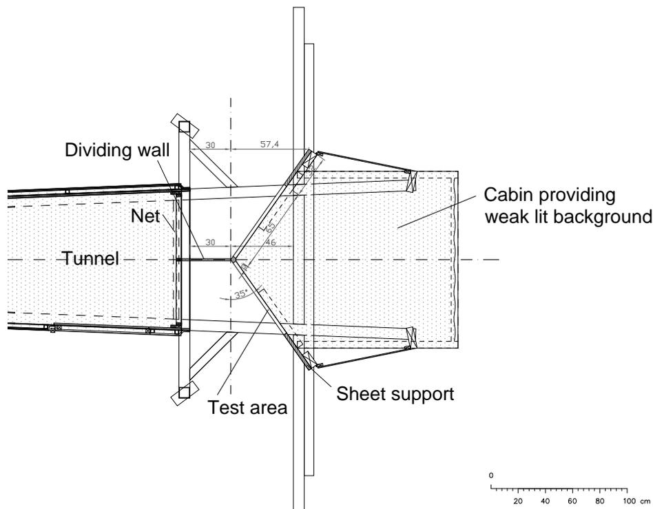
Figure 4: Horizontal section through the flight tunnel in the WIN test configuration with enclosed chamber (simulation of indoor rooms) behind the test panes positioned diagonally to the birds' flight axis.
