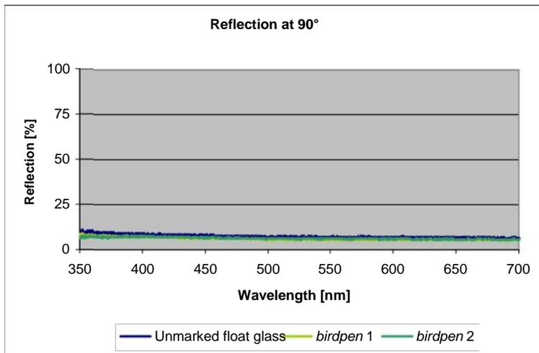
Figure 16: Spectral reflection on unmarked float glass (blue) and float glass with *birdpen* coating (greens). The measurement indicates generally low contrasts, which are slightly stronger in the UV spectrum than in the spectral range >400 nm
