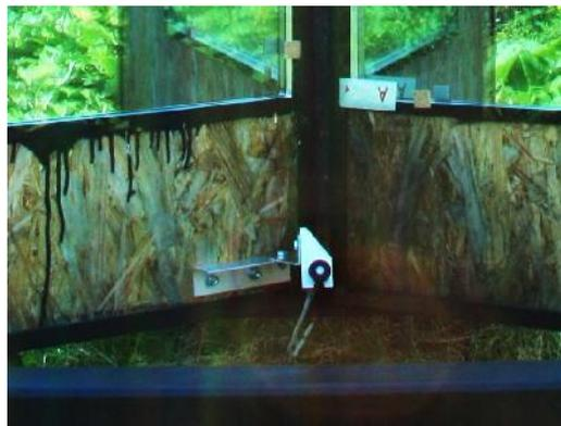
Figure 6: Photovoltaic sensor for measuring radiation behind the test panes.
