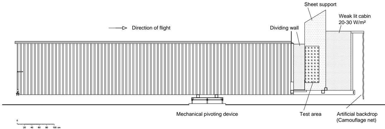
Figure 3: Flight Tunnel in the WIN test configuration. A ceiling, side walls and a partially translucent curtain create a weak-lit cabin behind the test panes. The trapezoidal sheet support prevents birds from seeing the sky and vegetation other than as reflections in the test area.
