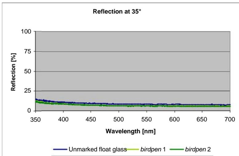
Figure 17: Spectral reflection on unmarked float glass (blue) and float glass with *birdpen* coating (greens). The measurement indicates generally low contrasts, which are slightly stronger in the UV spectrum than in the spectral range >400 nm
