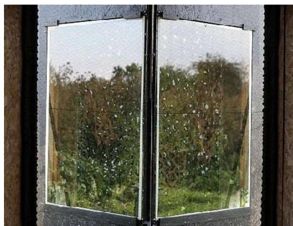
Figure 13: WIN reference test – *birdpen* vs. unmarked float glass. Unmarked float glass on the left (reference), test pane on the right (*birdpen* on float glass).
