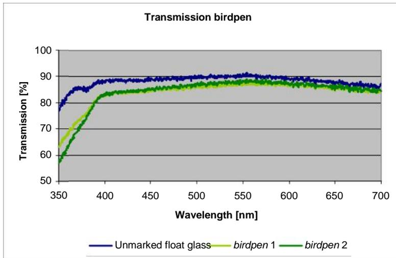
Figure 15: Spectral transmission through unmarked float glass (blue) and float glass with *birdpen* coating (greens). Stronger UV absorption of *birdpen* is clearly apparent. In the practical application as a window marking, however, UV absorption from background light is irrelevant, since UV is not emitted from inside buildings.
