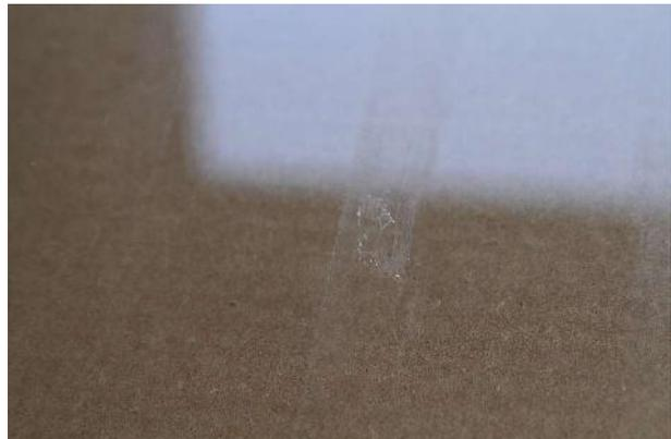
Figure 9: When turned into the light or backlit, adhesive residue-like streaks become visible.
