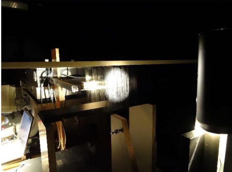
Figure 7: Spectral measurement, in this case of the transmission properties, of a large-surface *birdpen* coating. Right: light source, centre: illuminated *birdpen* coating, left: sensor of the spectrometer behind the pane. The test pane is oriented with computer-controlled servomotors.
