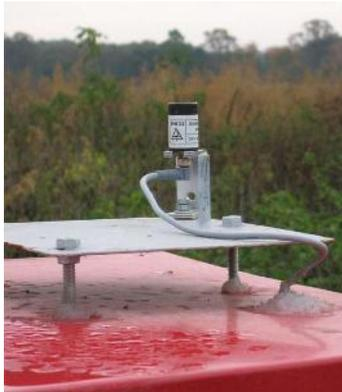
Figure 5: Photovoltaic sensor for measuring global radiation.
