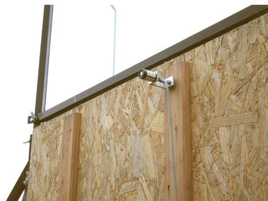
Figure 8: Pyranometer 1 for measuring global radiation
